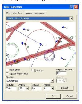
See You users go to Task Properties and enter the barrel size in radius 1 and 180° in the angle box. At its simplest the task can be flown by turning as soon as the GPS distance from the goal is less than the given barrel size.
