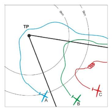
In this example highest handicap glider A rounds the task turn point. Lower handicap glider B has been given a barrel size of 6 km and the lowest handicap glider C has a barrel size of 9km. The distance handicap keeps the gliders in proximity throughout the task.
